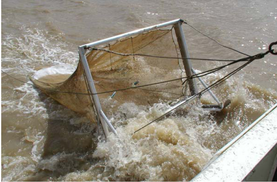
Figure 7: Detailed view of the Agassiz trawl.
