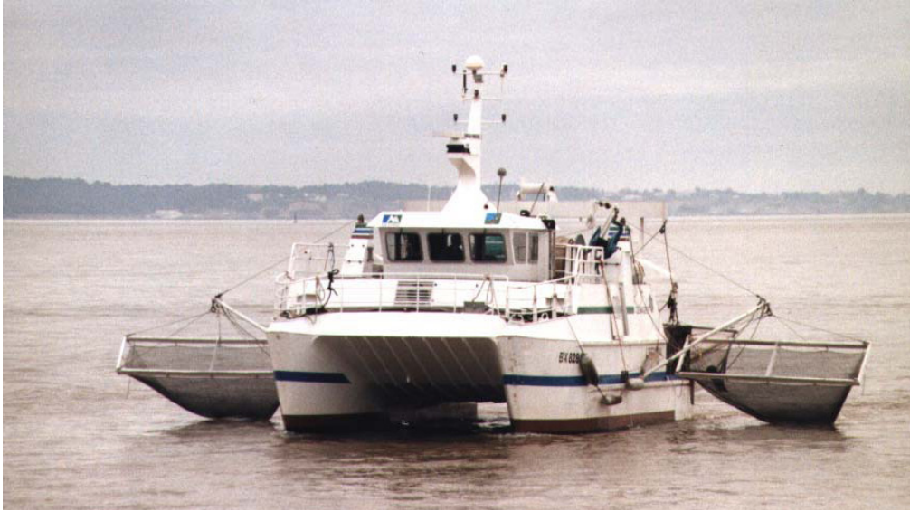
Figure 5: The estuarine research vessel fitted equipped with two push-nets (out of the water)
