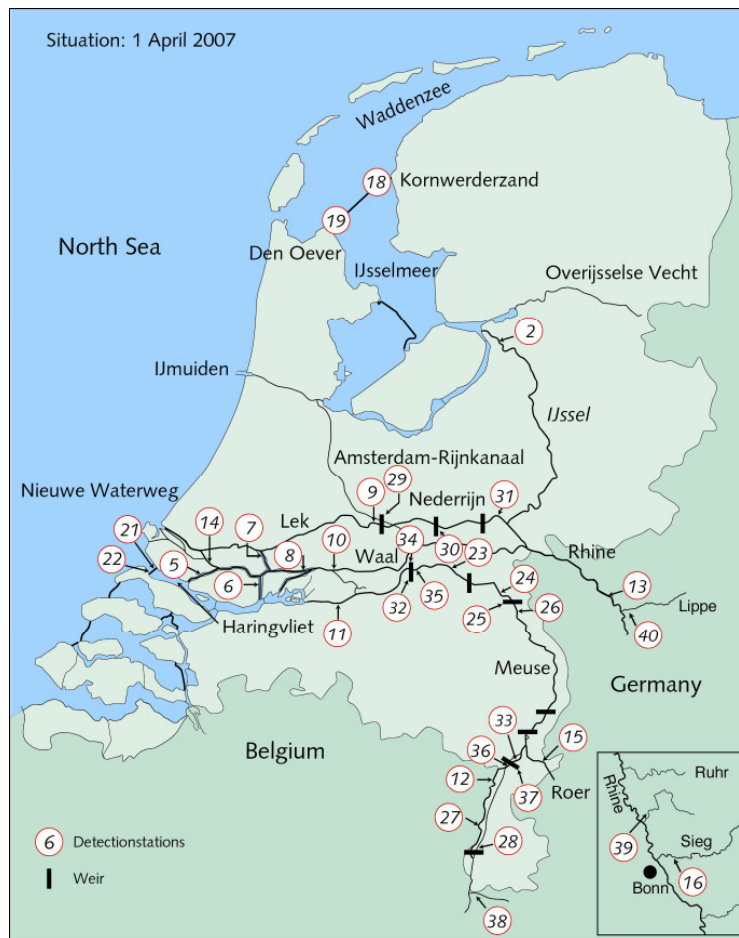
Figure 16: Fixed detection stations for NEDAP trail transmitters in the branches of the Dutch Rhine and Meuse delta and the lower parts of the Meuse and the German Rhine as well as its major tributaries in North Rhine-Westphalia allow to tracing the routes of up- and downstream migrating fish equipped with the respective transmitters. In the future the NEDAP system could even provide information on the migration routes of adult Allis shads.
